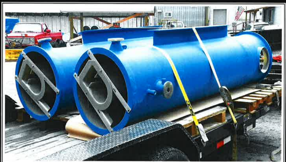
3' Water Filtration Tanks
