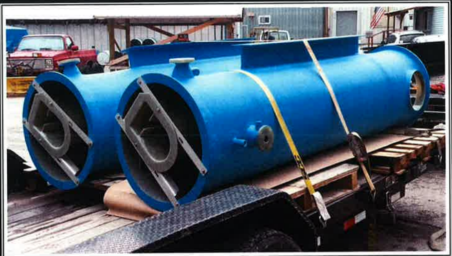
3' Water Filtration Tanks
