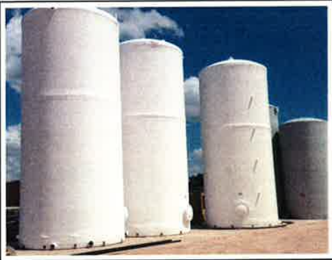
14' Diameter Vertical Chemical Storage Tanks
