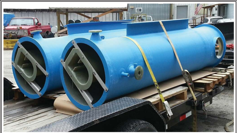
3' Water Filtration Tanks
